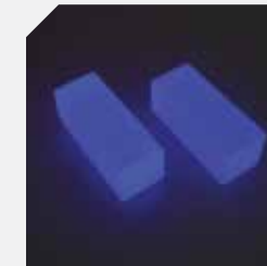
CLYC scintillator crystals under UV excitation Radiation Monitoring Devices, Inc.
