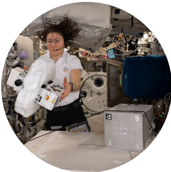
NASA astronaut Christina Koch onboard the ISS with Orbit Fab's FlexTank™ (left) and the rigid tanker (right) during testing.
