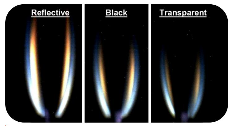
This image shows flames during the confined combustion experiment, which used simulated walls with reflective, black, and transparent treatments to study how flames behave in different types of confinement.
