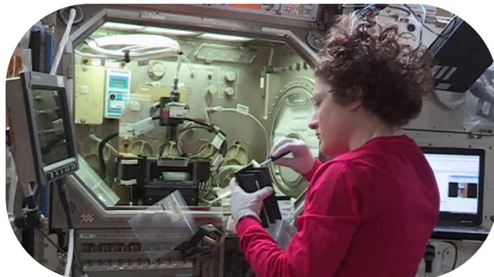
*NASA astronaut Christina Koch installs samples for experimental burning in the Microgravity Science Glovebox during the confined combustion investigation onboard the space station.*
