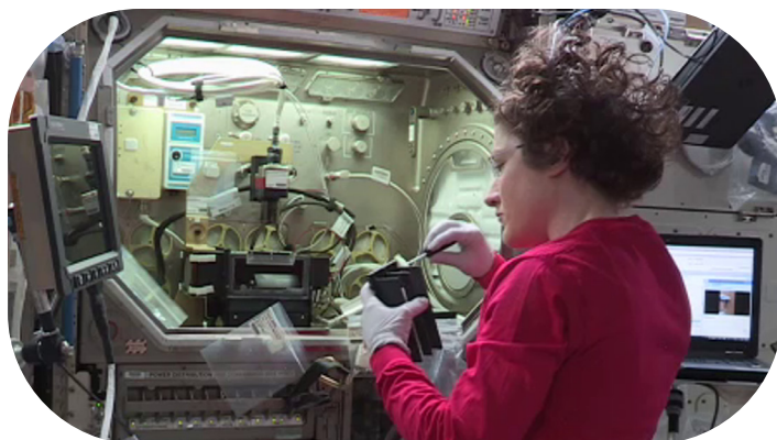
NASA astronaut Christina Koch installs samples for experimental burning in the Microgravity Science Glovebox during the confined combustion investigation onboard the space station.
