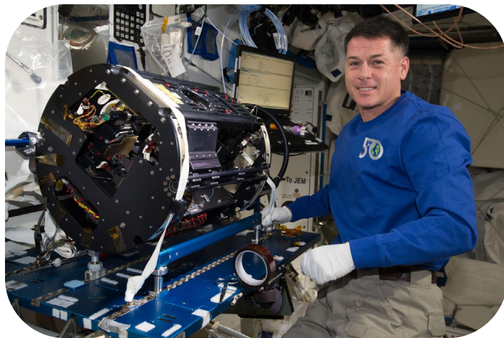
NASA astronaut Shane Kimbrough completing the Multi-user Droplet Combustion Apparatus reconfiguration for the cool flames investigation setup.
