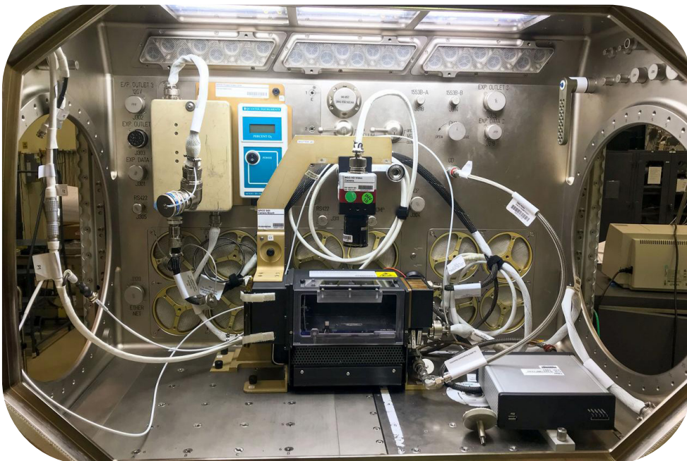
The configuration of the Microgravity Science Glovebox for the confined combustion experiment is shown here before launch.
