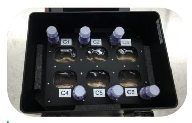
A view of the biocell that housed the heart cells on the space station.
