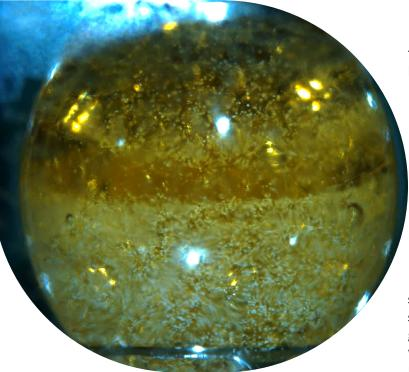
The Ring Sheared Drop system on the ISS containing a concentrated solution of human serum albumin, the main protein constituent of blood. Small white dots are glass tracer particles that allow researchers to study fluid flow of biofluids in space. Joe Adam
