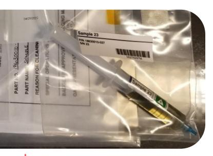
Protein solution sample for the investigation loaded into a syringe for launch to the ISS.
