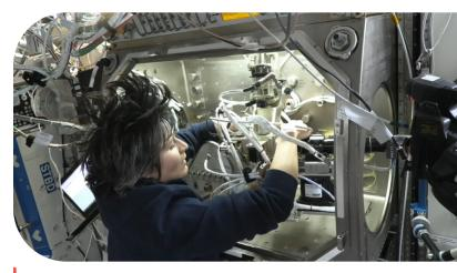
ESA astronaut Lt. Samantha Cristoforetti installing the Ring Sheared Drop system into the Microgravity Science Glovebox on the ISS. NASA
