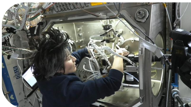
**ESA astronaut Lt. Samantha Cristoforetti installing the Ring Sheared Drop system into the Microgravity Science Glovebox on the ISS.**
