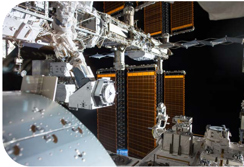
The NREP being translated to the Japanese Experiment Module Exposed Facility by the Japanese Robotic Arm.
