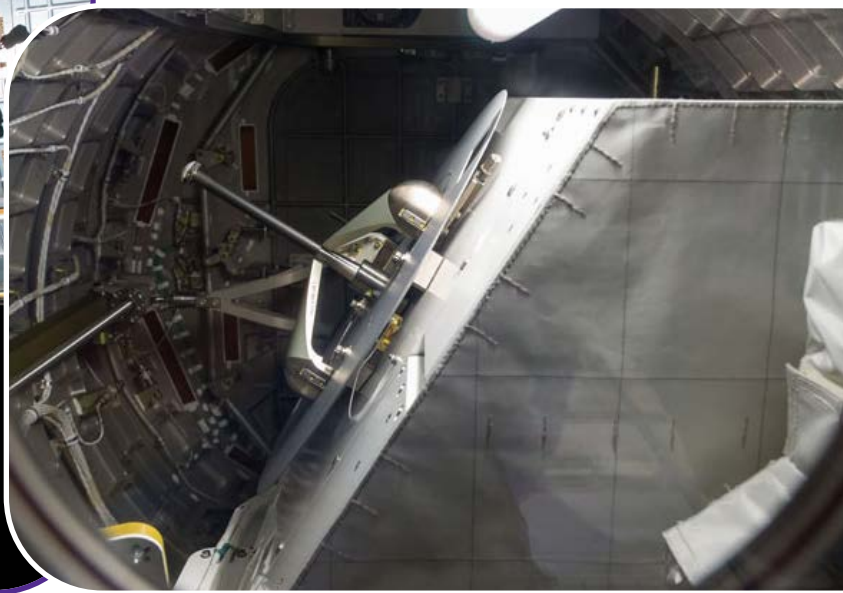
The NREP inside the Japanese Experiment Module airlock. Payloads are installed inside the pressurized volume of the ISS, and then the NREP and payloads are transferred outside and installed on the Japanese Experiment Module Exposed Facility.
