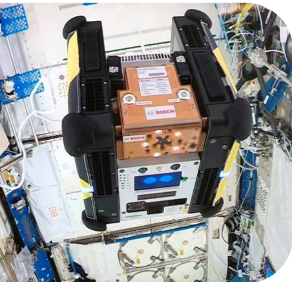
The SoundSee system installed on an Astrobee on the space station.
