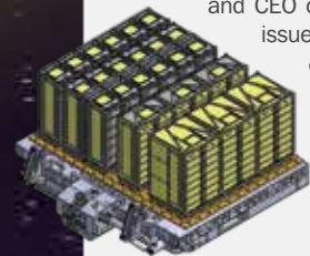
Computer-aided design image of the RM3S Deployer, designed with the purpose of deploying nanosatellites and microsattelites from the ISS LaMont Aerospace
