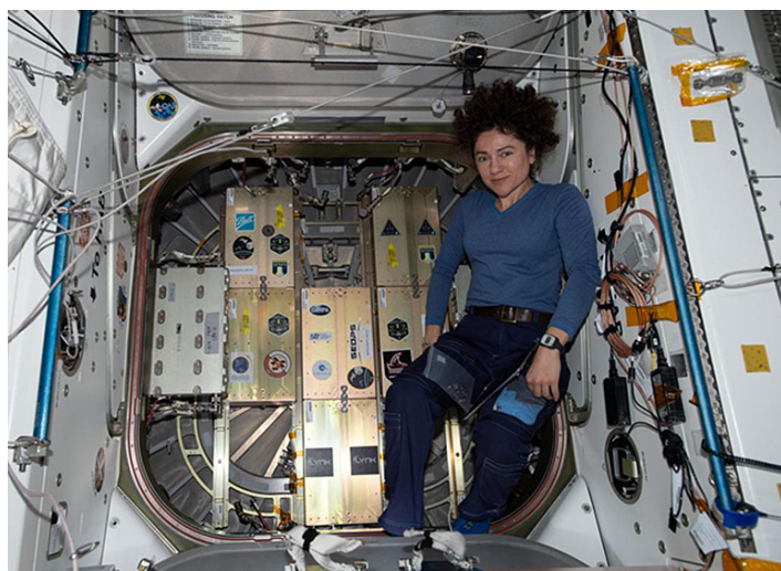
NASA astronaut Jessica Meir poses in front of the closed hatch of the Cygnus space freighter from Northrop Grumman. Attached to the hatch is the SlingShot smallsat deployer loaded with eight CubeSats that were deployed into Earth orbit for communications and atmospheric research several hours after Cygnus departed the orbiting lab on Jan. 31, 2019.
