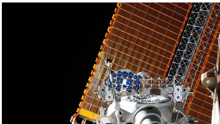
The MISSE Flight Facility is a permanent in-orbit platform from Alpha Space Test and Research Alliance that is mounted externally on the space station.
