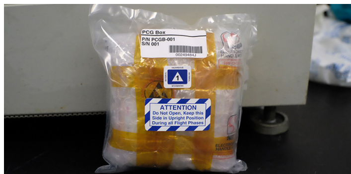
The Toledo Crystallization Box (TCB) shown here is packed with 50 individual crystallization experiments and ready for flight.
