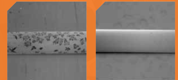
Scanning electron microscope images of ZBLAN fibers: at left, processed in unit gravity forming visible crystals; at right, processed with magnetic eliminating crystal formation. NASA
