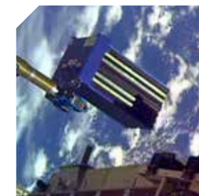
Robotic transfer of the MISSE-9 MISSE sample carriers from the JEM Airlock to the MISSE-FF on ELC-2. NASA
