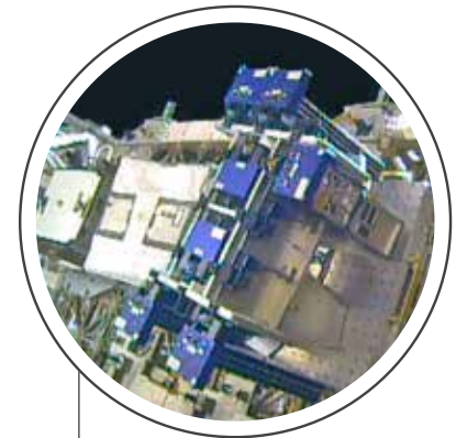
MISSE-FF with the zenith MISSE sample carrier open and the samples exposed to space. NASA
