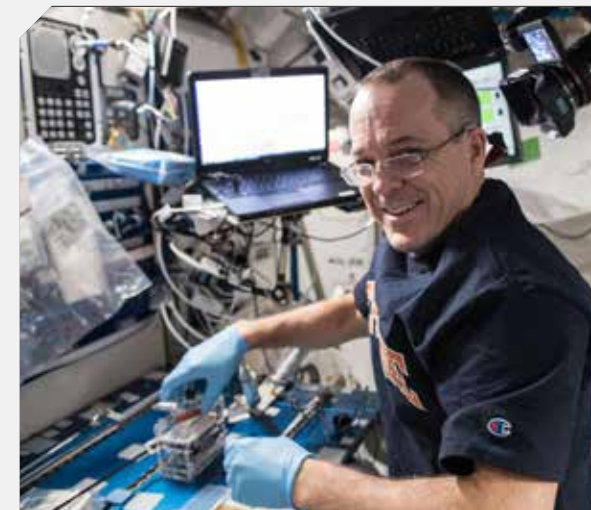
NASA astronaut Ricky Arnold swabbed surfaces in the ISS to collect microbe samples and then processed the microbial DNA using the Biomolecule Sequencer, a device that enables DNA sequencing in microgravity, to identify microbes able to survive in microgravity.
