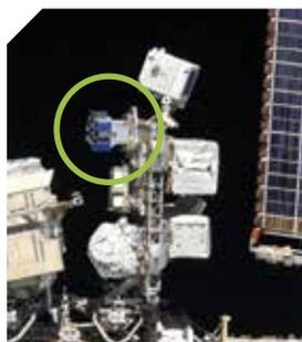
*The MISSE-FF platform, developed by Alpha Space, on the ISS.*
