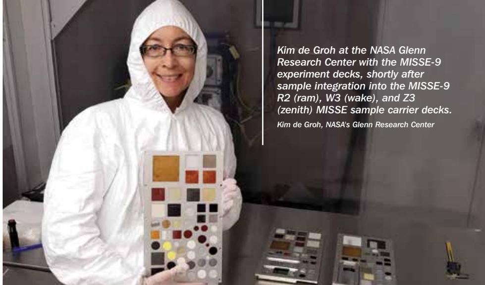
Kim de Groh at the NASA Glenn Research Center with the MISSE-9 experiment decks, shortly after sample integration into the MISSE-9 R2 (ram), W3 (wake), and Z3 (zenith) MISSE sample carrier decks.
