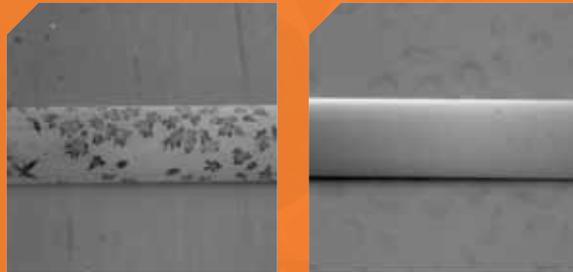
Scanning electron microscope images of ZBLAN fibers: at left, processed in unit gravity forming visible crystals; at right, processed with magnetic eliminating crystal formation. NASA
