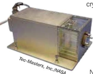
During Ostrogorsky's first SUBSA experiments in 2002, melting and directional solidification was observed for the first time under microgravity conditions. A data downlink from the video-enabled furnace on the ISS allowed Ostrogorsky to coordinate with NASA Astronaut Peggy Whitson to change temperatures, melt times, and other factors, observing how they affected crystallization. These experiments facilitated better understanding of the complex effects of convection in crystallization.
