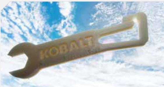
*A space-optimized wrench for ISS crew members 3D-printed onboard the space station using the Additive Manufacturing Facility.*
