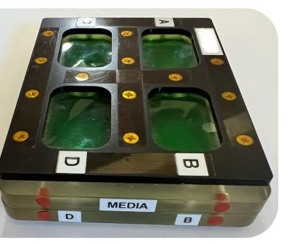
BioServe's four-well dual chamber BioCell hardware BioServe Space Technologies
