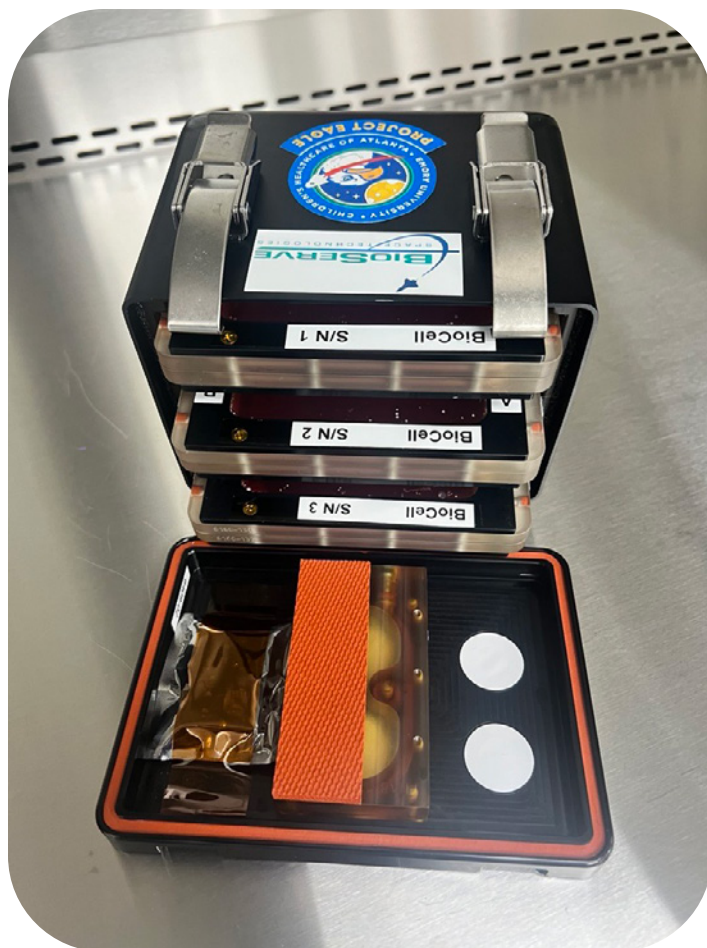
Cardiac muscle cell samples loaded into BioServe's BioCell hardware for Project Eagle.
