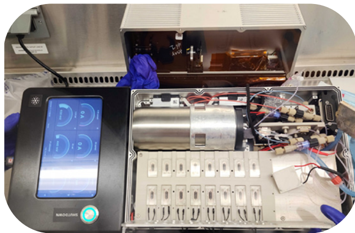
The 16 human skeletal muscle tissue chips integrated into a CubeLab for an experiment on the ISS. Half of the tissue chips contain electrodes to deliver electrical stimulation to induce contraction in the myobundles.
