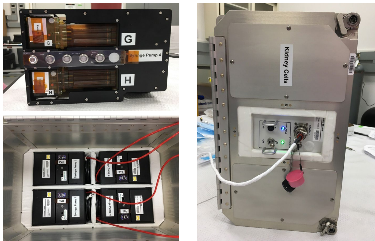
Figure 8: Showing the final hardware configuration for the Kidney Chips in Space ISS payload. The configuration reduced a conventional laboratory setup requiring four syringe pumps, two incubators, and >30.5 m of tubing and a total volume of ~ 1,350 L down to a final installed volume on the ISS of just 45 L. Image courtesy of BioServe Space Technologies
