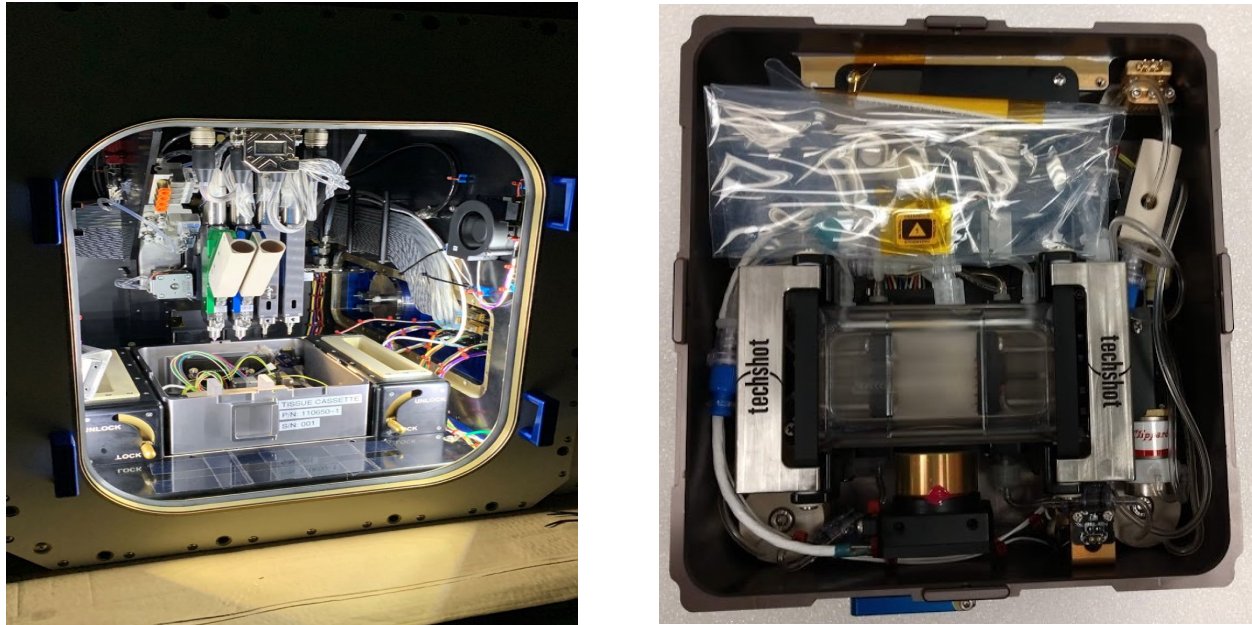
Figure 3: Left figure showing the inside of the BFF, specifically the bioprinter component that is capable of multicomponent printing using its four-independent-head design. Right figure is the tissue culture chamber that the printed material is moved to. Figures courtesy of Techshot, Inc.
