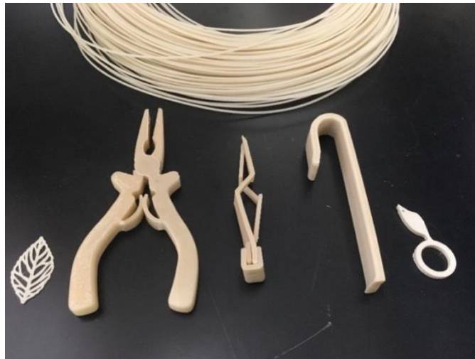
Figure 5: Articles produced from Mango's in-house, 3D-printed PHA polymers. Courtesy of Mango Materials
