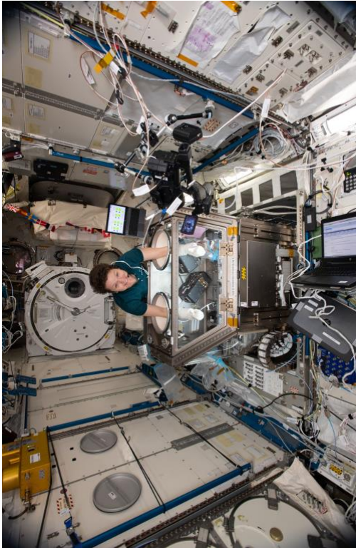
Fig. 2. NASA astronaut Anne McClain works inside the Life Sciences Glovebox with the Tissue Chips in Space Kidney Cells investigation. Image Credit: NASA
