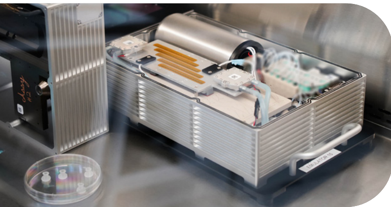
A flight-ready CubeLab, integrated with Encapsulate's biochips and microfluidic device for cancer research, is tested preflight on Space Tango's emulator.
