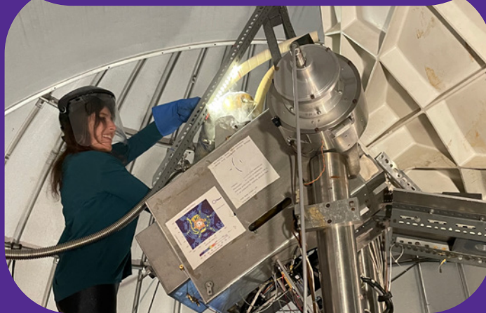
Kaylie Hausknecht fills a dewar with liquid nitrogen at the Harvard-Smithsonian Center for Astrophysics 1.2-meter telescope.
