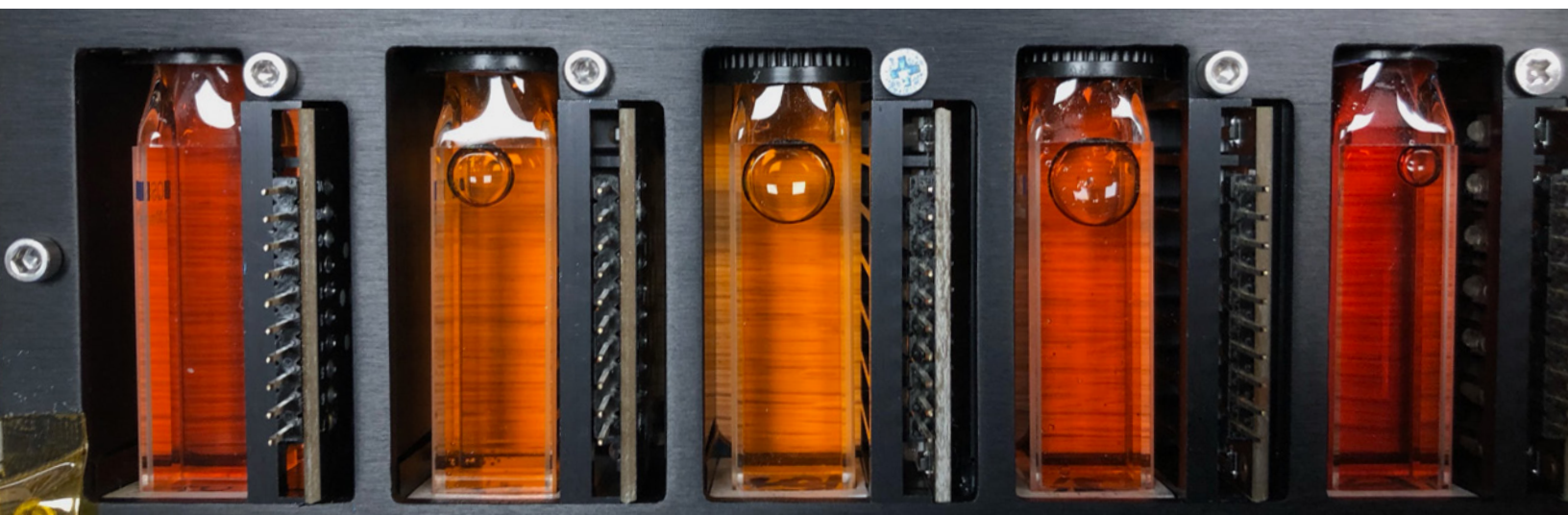
Five fluid-filled cuvettes prepared for launch to the ISS as part of the investigation.
