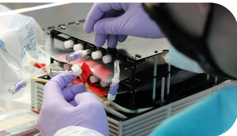
*Deintegration of a CubeLab containing LambdaVision’s artificial retinas produced in microgravity.*
