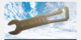
A space-optimized wrench for ISS crew members 3D-printed onboard the space station using the Additive Manufacturing Facility. Made In Space ISS that requires optimal resource allocation. The ability to reuse plastic items and transform them into feedstock without need for terrestrial resupply will mean less space required for raw material storage, as well as greater overall printing capacity to produce needed parts and tools.
