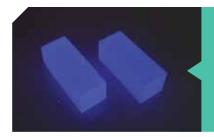
CLYC scintillator crystals under UV excitation Radiation Monitoring Devices Inc.
