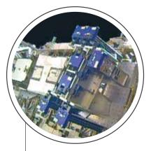
MISSE-FF with the zenith MISSE sample carrier open and the samples exposed to space. NASA
