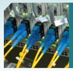
Fiber optic cables used in modern communication. ISS National Lab These optical fibers are most commonly made of silica (SiO<sub>2</sub>) glass. While silica fibers are easily produced using well-established methods, optical losses in the fiber requires the use of expensive repeaters to boost the signal across long transmission distances.
